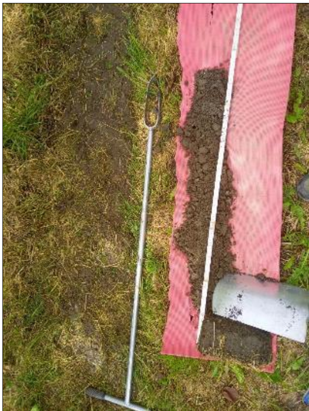
Photo 1 : Sondage T2 : horizons Ah (0 – 15 cm), AB (15 – 40 cm), B (40 – 70 cm) et Bg (70 – 75 cm)
